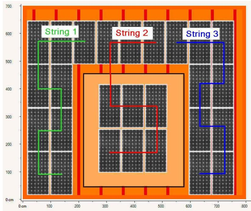
**Fig. 2: String connection of the 27 modules on an example string inverter (ESI)**
