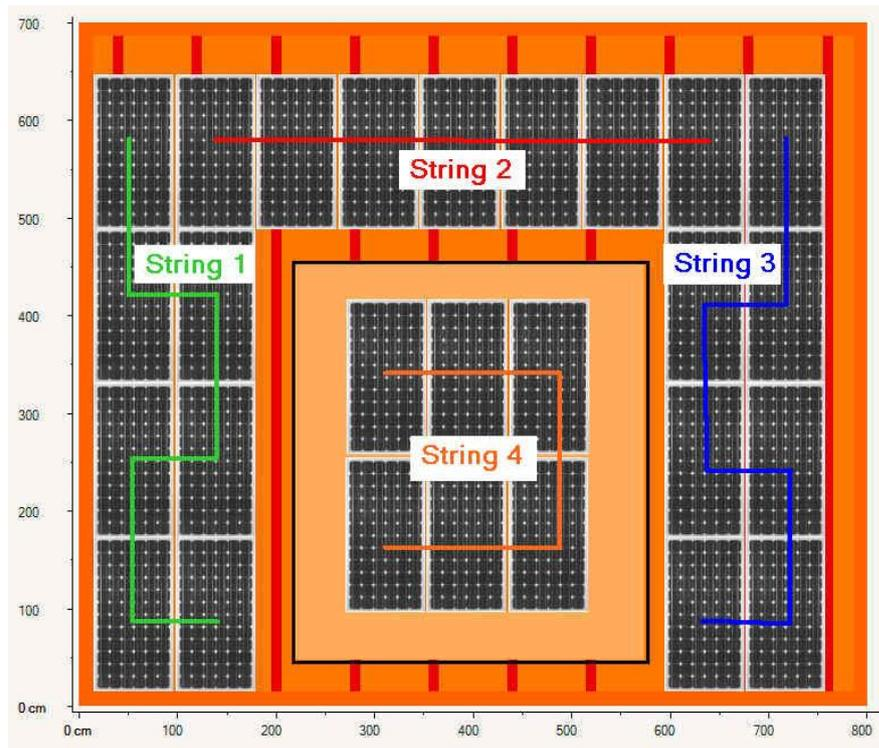
Fig. 3: String connection of the 27 modules on the StecaGrid 2000+ inverters
