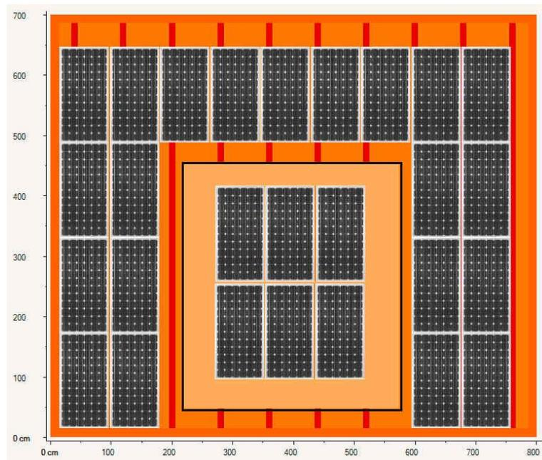
**Fig. 1: Distribution of the 27 PV modules on the surface of the specimen roof and the dormer**
